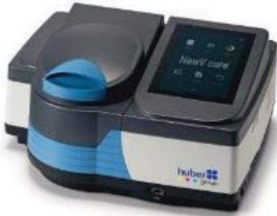
Prototype of the NewV cure device, which provides press operators with a fast, easy, and reliable way to determine UV cure of **hubergroup's** NewV inks.
